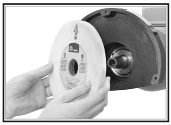
Figure 17. Removing wheel.
